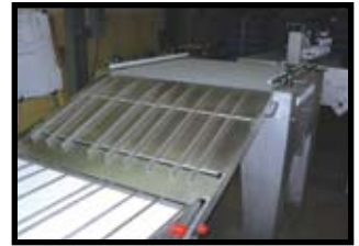
Accumulation Conveyor and Slide
